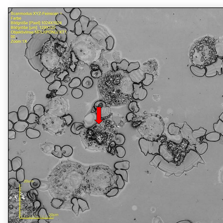
Fig. 11: Ashes. Ashing at 130 °C, for 48 Hrs. LEXT OLS2000. Original magnification x8545.
